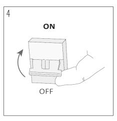
Be sure the installation is done right before switching ON the fuse.
