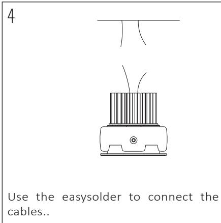
Use the easysolder to connect the cables..
