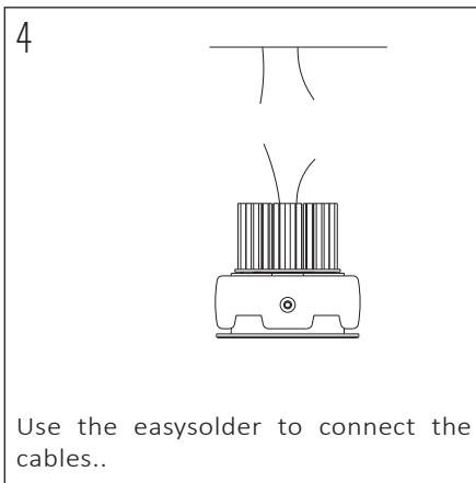
Use the easysolder to connect the cables..
