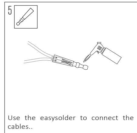
Use the easysolder to connect the cables..
