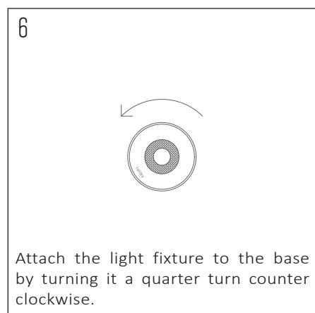
Attach the light fixture to the base by turning it a quarter turn counter clockwise.
