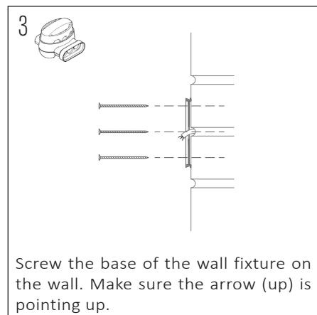
Screw the base of the wall fixture on the wall. Make sure the arrow (up) is pointing up.
