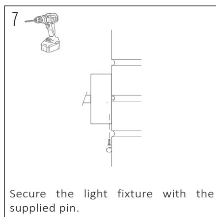
Secure the light fixture with the supplied pin.
