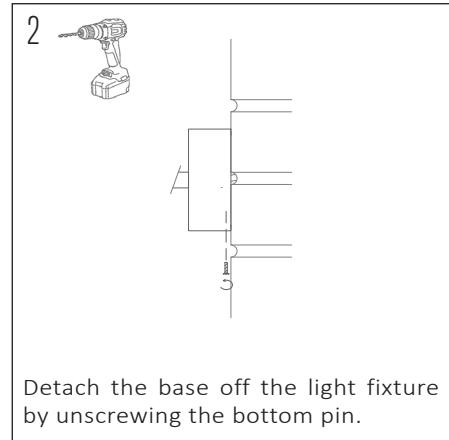
Detach the base off the light fixture by unscrewing the bottom pin.
