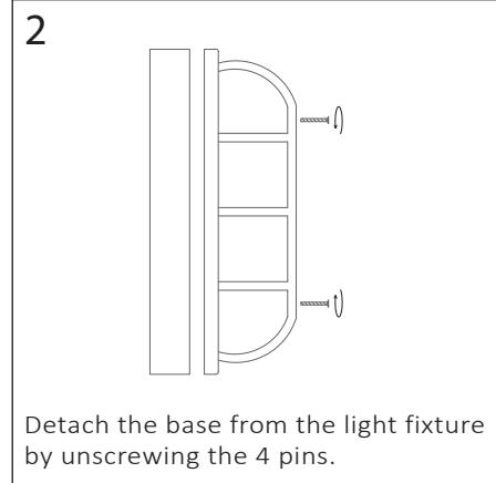
Detach the base from the light fixture by unscrewing the 4 pins.
