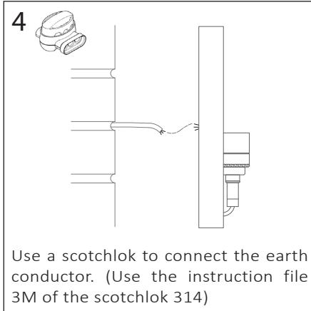
Use a scotchlok to connect the earth conductor. (Use the instruction file 3M of the scotchlok 314)
