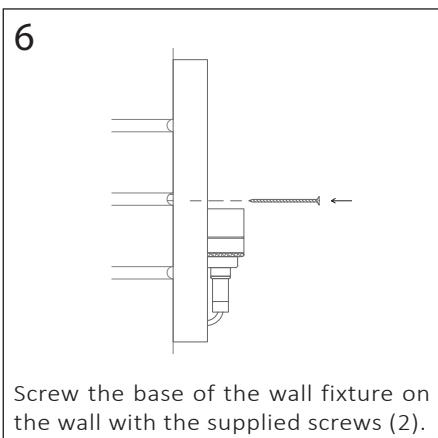
Screw the base of the wall fixture on the wall with the supplied screws (2).
