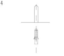
Use a hammer to install the screw plug in the drilled holes.
